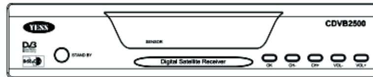
**STAND BY :** Press to switch between operation and standby modes
